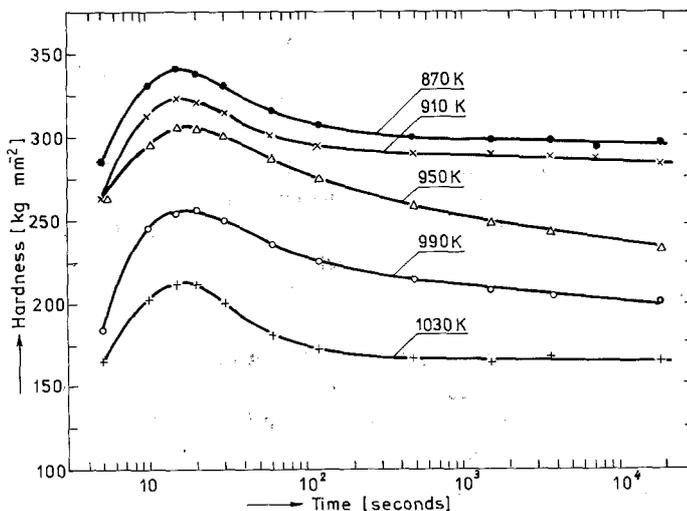
Figure 1 Hardness isotherms of the CuNiCo alloy.
