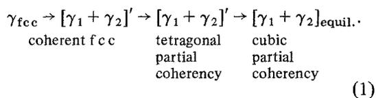
The decomposition products are parallel to the  $\{100\}$  matrix surface and in the final state, in the late ageing stages, the  $\gamma_1$ -phase is NiCo-rich and the  $\gamma_2$ -phase is Cu-rich. In the alloy with optimum magnetic properties the ferromagnetic  $\gamma_1$ -phase particles are close to the critical size required to be single domains.
